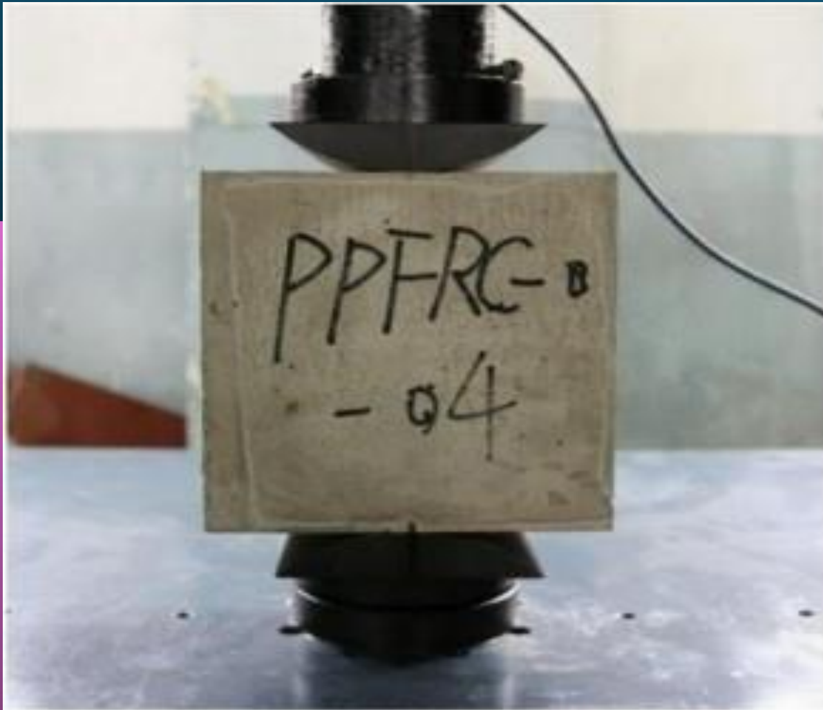
(a) Placement of concrete specimen
